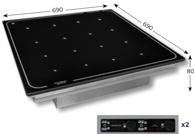
Product cut-out dimensions: 696 x 696 mm Control panel cut-out dimensions: 390 x 88 mm
