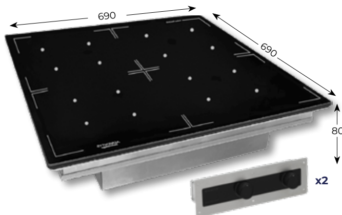
Product cut-out dimensions: 696 x 696 mm Control panel cut-out dimensions: 392 x 80 mm
