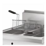
In the gas version, the burner is outside the tank, is made with stainless steel and has a stabilised flame. Piezoelectric ignition and safety ensured by a valve with a thermocouple and pilot flame.
