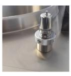
Indirect heating with low-pressure steam generated by the water in the jacket: safe and easy operation thanks to pressure gauge, safety valve and compensating valve.
