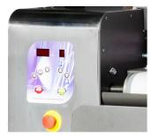
**ST23**ST23 control, standard on the entire gamma, manages temperature using the P.I.D. system (Proportional - Integral - Derivative).
