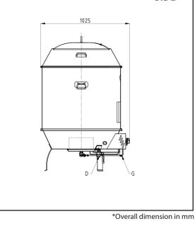
**TECHNICAL DATA External Dimensions** Width : Ø 936 mm : 1025 mm Depth Height : 1540 mm **Cooking Surface** Cooking zones : 12 ducks, Ø 900 mm
