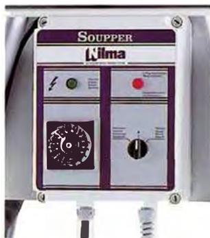
Low voltage control board (24 V.) equipped with: ON/OFF push button, manual/stop/automatic selector, flow programmer, power indicator and faulty connection light. Protection degree: IPX4.
