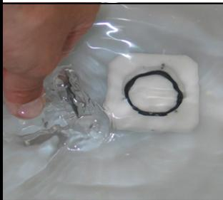
**5th:** Swish the nozzle in the remaining Sanitizing Solution (left over from the Sauce dispenser's Sanitize Cycle) to Rinse and Sanitize all Nozzle surfaces or, see *Solution Instructions* below to prepare Sanitizer solution in a sink.
