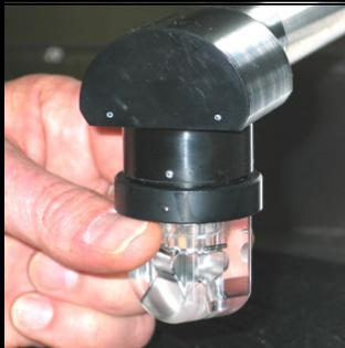
**1st:** Grasp and turn the nozzle Clockwise until the silver dots are aligned.
