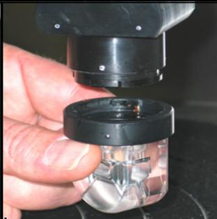
**2nd:** Pull the Nozzle down and away from the Nozzle Mount. Wash, Rinse, and Sanitize the Nozzle before re-using.
