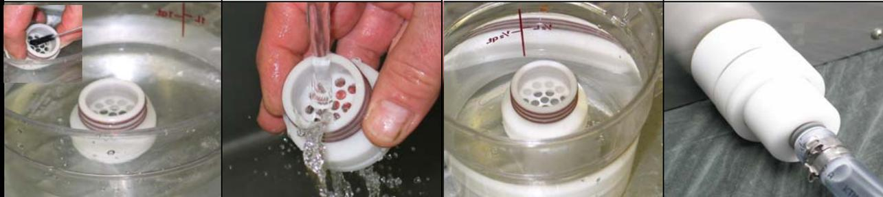
**5th:** Soak the Strainer in a clean container filled with Detergent Solution (page 7 *Detergent Solution*) for more than 2 minutes. Clean all holes with 1/4" Bristle Brush.
