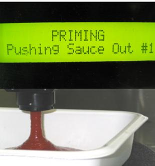
**11th:** The pump will fill and dispense 4 times and then stop. (Display will say: PRIMING Pushing Sauce Out #1, PRIMING Pushing Sauce Out #2, then #3, and then #4.
