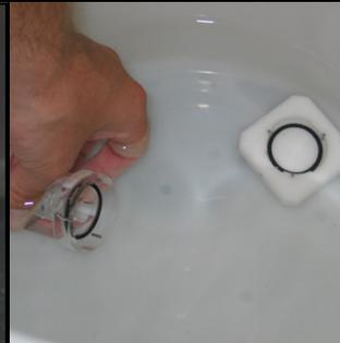
**3rd:** Place the Nozzle into detergent solution remaining from the Sauce dispenser's WASH cycle for 5 to 15 minutes or, see *Detergent Solution Instructions* below to prepare detergent solution in a sink.
