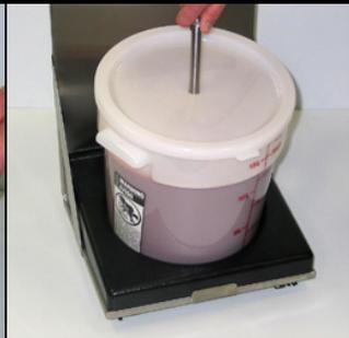
**4th:** Insert the Dip Tube thru the hole in the cover so that the Dip Tube end is oriented toward the front or lowest side of the Vat.
