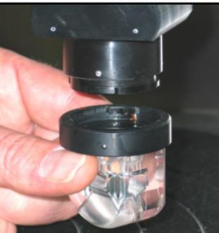
**10th:** Pull the Nozzle down and away from the Nozzle Mount. Wash, Rinse, and Sanitize the Nozzle before re-using.
