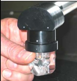
**9th: (Remove Priming Nozzle if used)** Install Nozzle : Grasp and turn the nozzle
