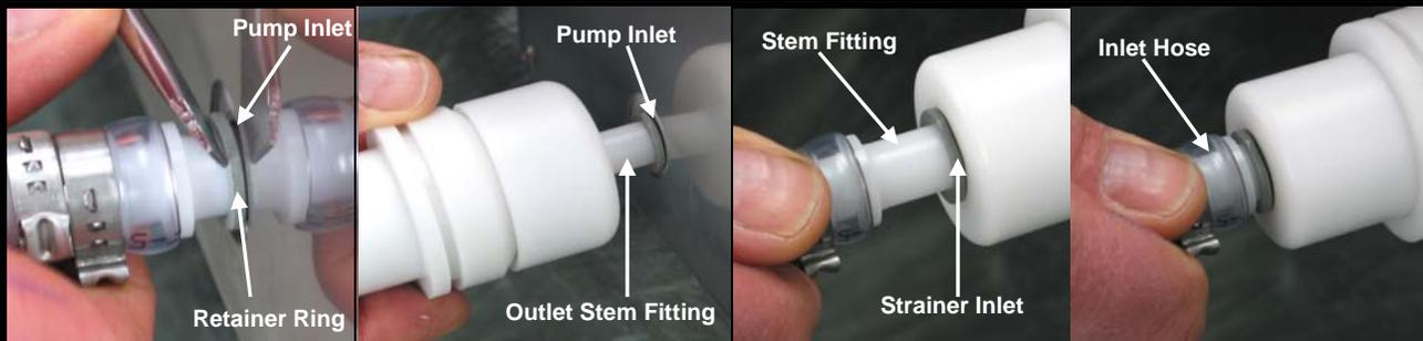
**1st:** Disconnect the Inlet Hose from Pump Inlet (lower back left of the pump enclosure) using a flat blade screwdriver to hold the gray retainer ring IN while pulling the fitting OUT.
