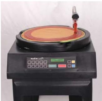
When the pizza dough is placed onto the turntable and the dispense button is pressed, the ready-to-use sauce is pulled into the pump chamber. It then travels up and into the sauce dispensing arm. The arm moves across the spinning pizza and dispenses the sauce in spiral pattern. Perfectly sauced pizzas at the touch of a button!
