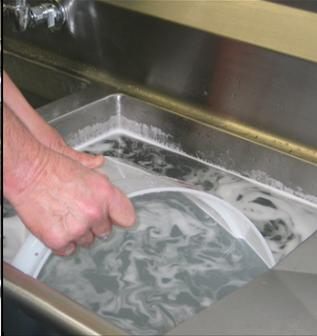
**7th:** Sanitize the Vat and Cover in the right sink. The right sink should contain warm water and Sanitizing solution. See *Sanitizing Solution Instructions* below.
