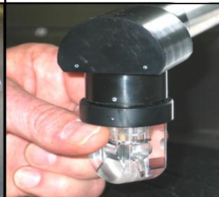
**7th:** Install the nozzle so that the silver dots are aligned.
