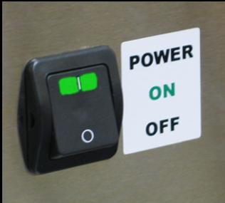
**5th:** Confirm that the Main Power Switch is ON. The Main Power Switch is located on the upper right side of the back splash.
